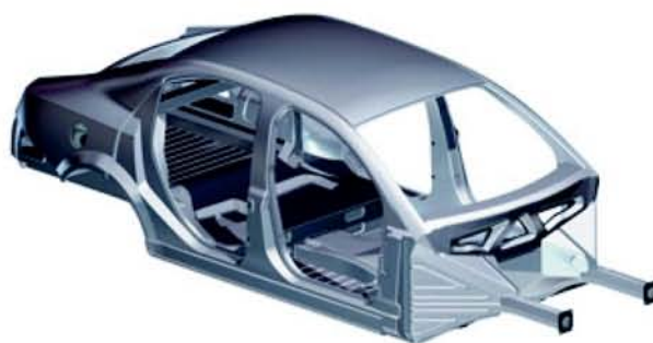
Figure 5: ULSAB-AVC Bodies-In-White; top shows C-Class (mass = 202 kg/445 lbs.); bottom shows PNGV-Class (mass = 218 kg/481 lbs.)
